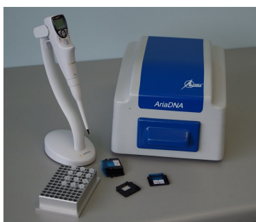
Microchip-based real-time PCR analyzer AriaDNA
