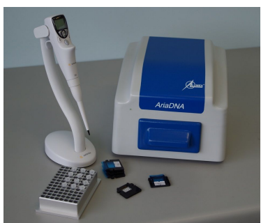
Microchip-based real-time PCR analyzer AriaDNA
